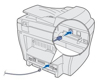
**2** Connect either a parallel (IEEE-1284 compliant) *or* USB cable to the printer port and the other end to your computer.
